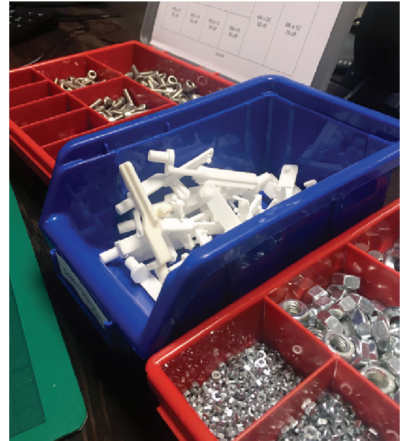
Selective Laser Sintered nylon spare parts.
